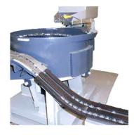
**Feeding Concepts Bowl Feeders** Versatile vibratory bowl feeders and centrifugal feeders feed parts at very high rates with exceptional accuracy.
