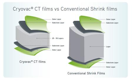
Innovative Technology 4 gauges from 30 to 70 gauge Sealed Air micro-layering technology Improved toughness Outstanding Benefits Enhanced tear resistance Soft shrink finesse films Excellent optics
